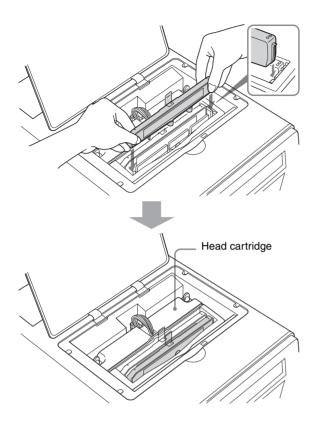
Load the remaining ink cartridges using the same procedure, matching the ink cartridge and its proper location.
